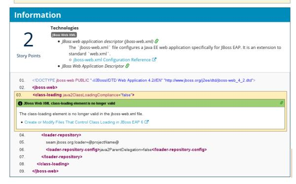
The top of the file lists the classifications for matching rules. You can use the link icon to view the details for that rule. Notice that in this example, the <code>jboss-web.xml</code> file matched on another rule (<code>JBoss web application descriptor (jboss-web.xml)</code>) that produced <code>1</code> story point. This, combined with the <code>1</code> story point from our custom rule, brings the total story points for this file to <code>2</code>.
